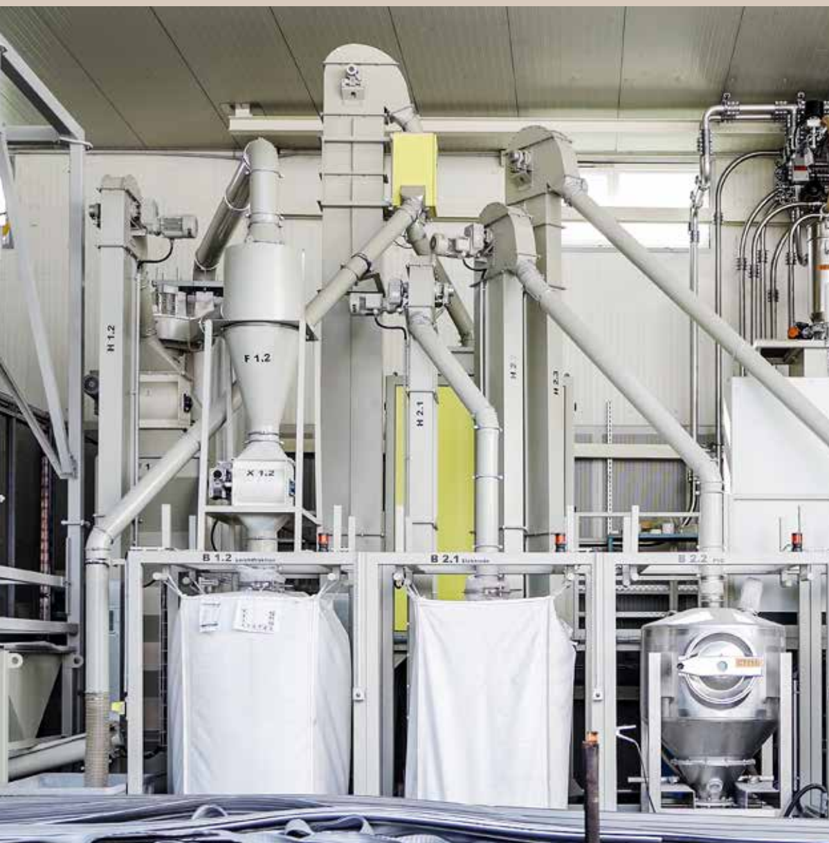
The modern recycling plant ensures the in-house reuse of all reject bars and offcut from the uPVC profiles produced by the company.
