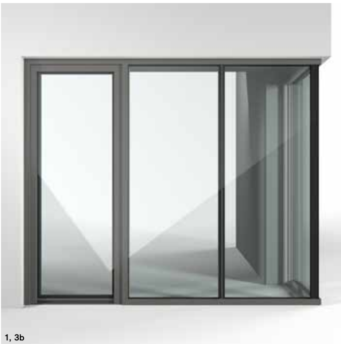
Window wall incorporating frameless casement door, three fixed lights with glass-covered mullion plus an all-glass corner (90°), faced on the interior with an aluminium angle
