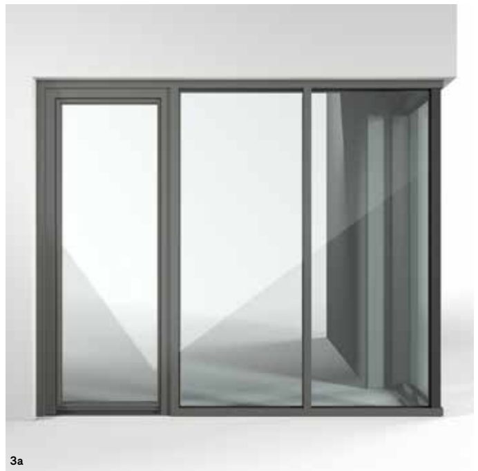
Window wall incorporating casement door plus three fixed lights and a glass corner (90°-150° possible), faced on the exterior with an aluminium angle
