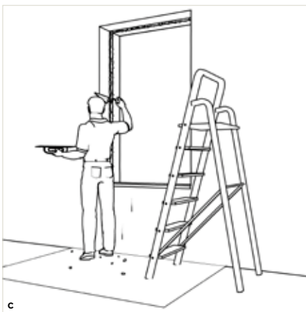
The reveal is made good on the inside and outside (by plastering/ rendering and painting). Scaffolding is used where necessary.
